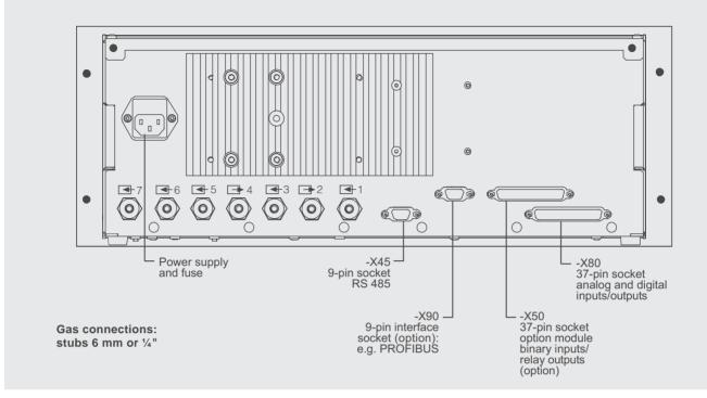
ULTRAMAT 23, 19" unit, e.g. one infrared component with oxygen measurement
