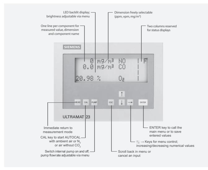
ULTRAMAT 23, membrane keypad and graphic display
