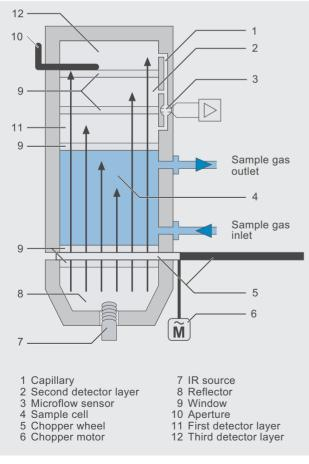
ULTRAMAT 23, mode of operation of infrared channel (example with three-layer detector)
