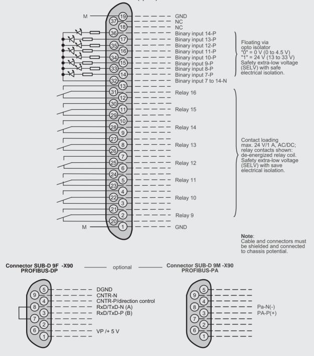
ULTRAMAT 23, pin assignment of the optional PROFIBUS interface board
