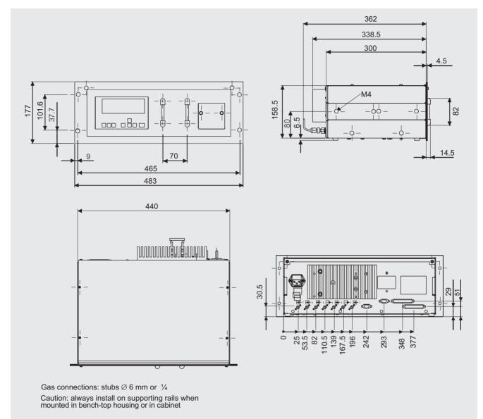
ULTRAMAT 23, 19" unit, dimensions in mm
