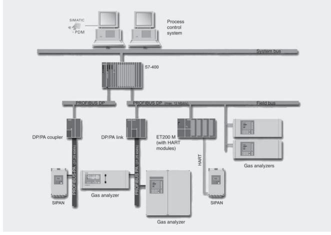
Basic structure of a PROFIBUS system
